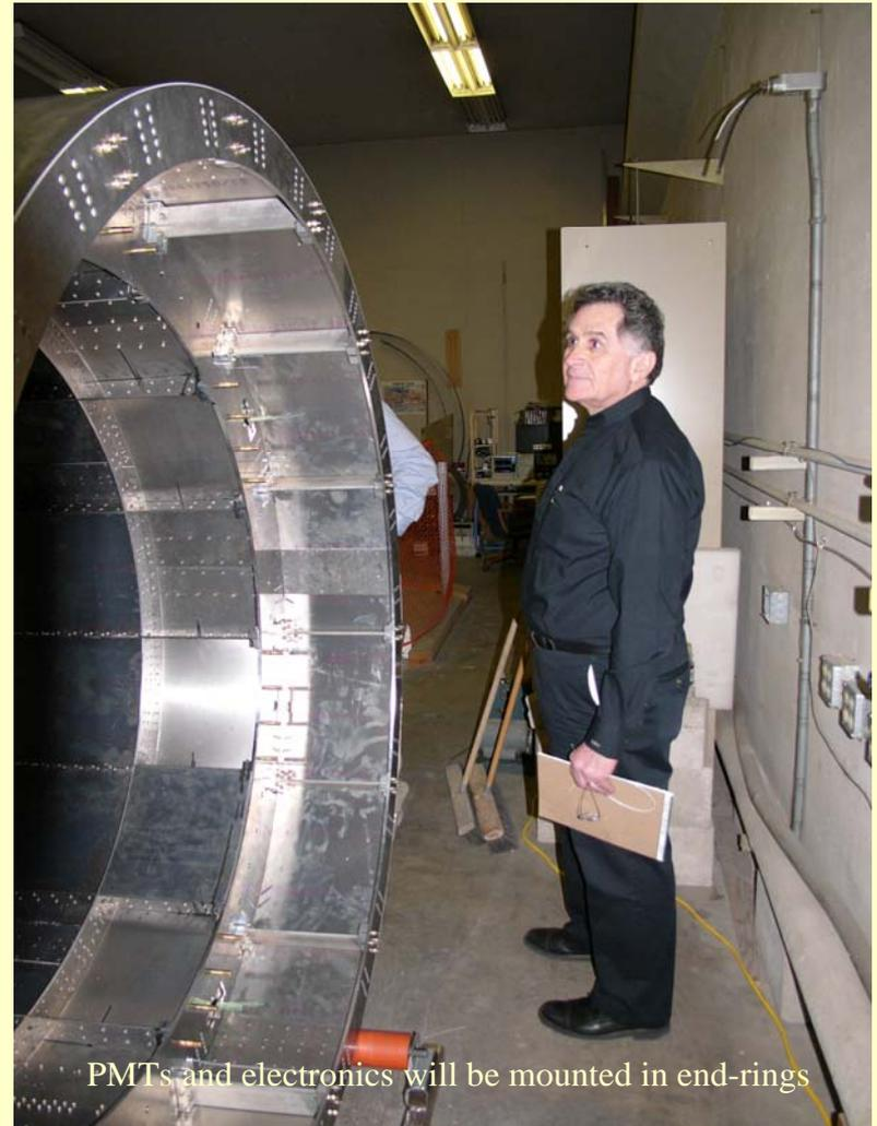
PMTs and electronics will be mounted in end-rings
