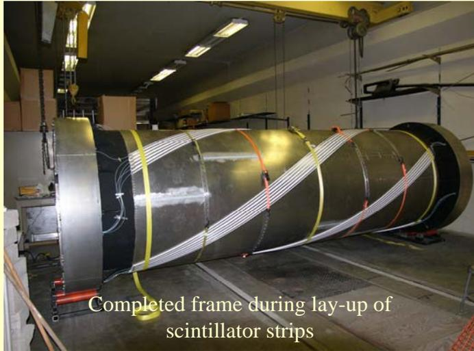
Completed frame during lay-up of scintillator strips
