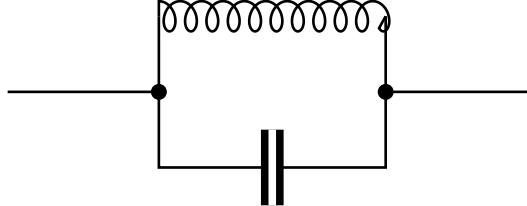
For simplicity, consider an ideal inductor (without any Ohmic resistance) and an ideal capacitor; a more realistic circuit will be the subject of a homework problem. Thus, the capacitor has impedance  $Z_C = 1/j\omega C$ , the inductor has impedance  $Z_L = j\omega L$ , and the whole parallel circuit has
