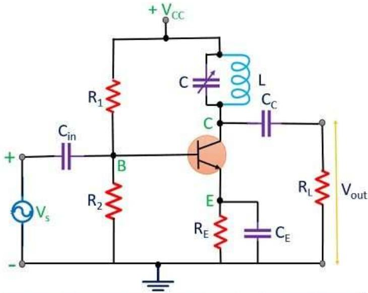
**Circuit of Single tuned amplifier with capacitive coupling**
