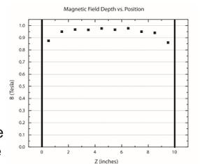
**Figure 6.** Preliminary measurements of field depth at various positions along the lens. The physical extent of the lens is indicated by the vertical lines at 0 and 10 inches.
