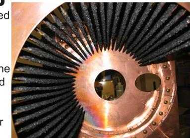
**Figure 4.** The cryosorption pump as seen from the helium nozzle. The inner and outer diameters of the barrel are 8" and 16", respectively. In this image, a number of the panels have been temporarily removed.
