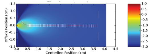
**Figure 1.** Shown above is the simulated average path of a lithium atom entering the jet having a given a particular initial velocity. White hash marks represent collisions with helium atoms. The background color represents the local temperature of the jet in Kelvin on a  $\log_{10}$  scale. The trajectory is calculated using a viscous damping model.
