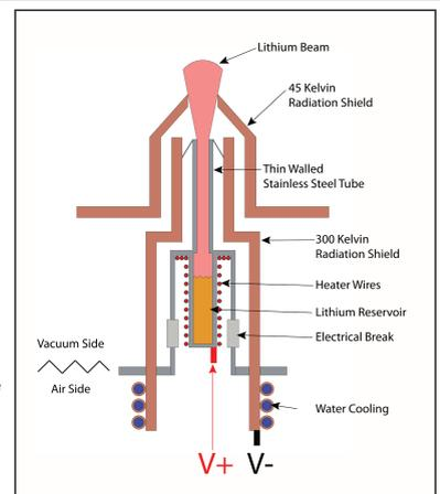
**Figure 5.** A schematic drawing of the lithium beam oven.
