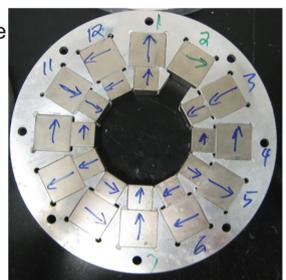
**Figure 7.** Shown above is a single layer of the lens. Magnetization directions of individual magnets are drawn on.
