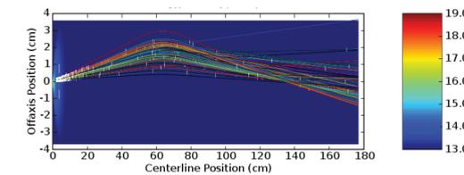
**Figure 2.** This plot shows trajectories of individual lithium atoms beyond the skimmer as they pass through the field of the hexapole lens. White hash marks indicate collision events with helium atoms. Each particle's flight is modelled using conventional Monte Carlo methods.
