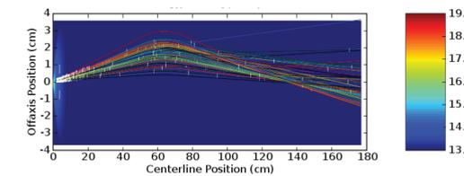
**Figure 2.** This plot shows trajectories of individual lithium atoms beyond the skimmer as they pass through the field of the hexapole lens. White hash marks indicate collision events with helium atoms. Each particle's flight is modelled using conventional Monte Carlo methods.
