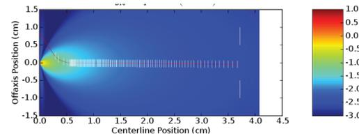
**Figure 1.** Shown above is the simulated average path of a lithium atom entering the jet having a given a particular initial velocity. White hash marks represent collisions with helium atoms. The background color represents the local temperature of the jet in Kelvin on a  $\log_{10}$  scale. The trajectory is calculated using a viscous damping model.
