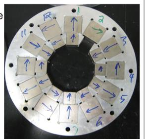
**Figure 7.** Shown above is a single layer of the lens. Magnetization directions of individual magnets are drawn on.
