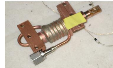
**Figure 3.** A picture of the 5 Kelvin anchored section of the helium source. The helium is cooled from 45 Kelvin to 5 Kelvin as it passes through the helical coil. A thermal sensor can be seen just atop the nozzle itself.
