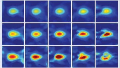
in a single step. As these pulses propagate through the medium they interact with the evolving object, and are imprinted with a 'phase streak' via cross-phase modulation in the process. The pulses are then simultaneously detected by a chargedcoupled device detector in a spectrometer. Finally, a modified tomography algorithm is used to generate movie frames of the object moving through the medium.
