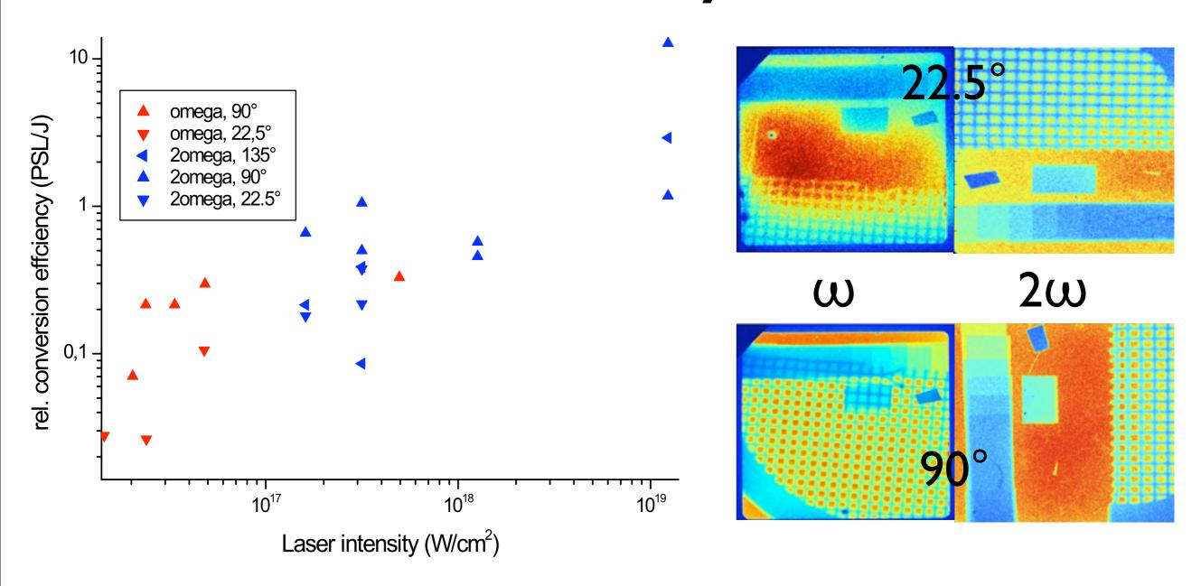
Frequency doubling can improve a lot at small incidence angles. Effect has not been observed for higher photon energies
