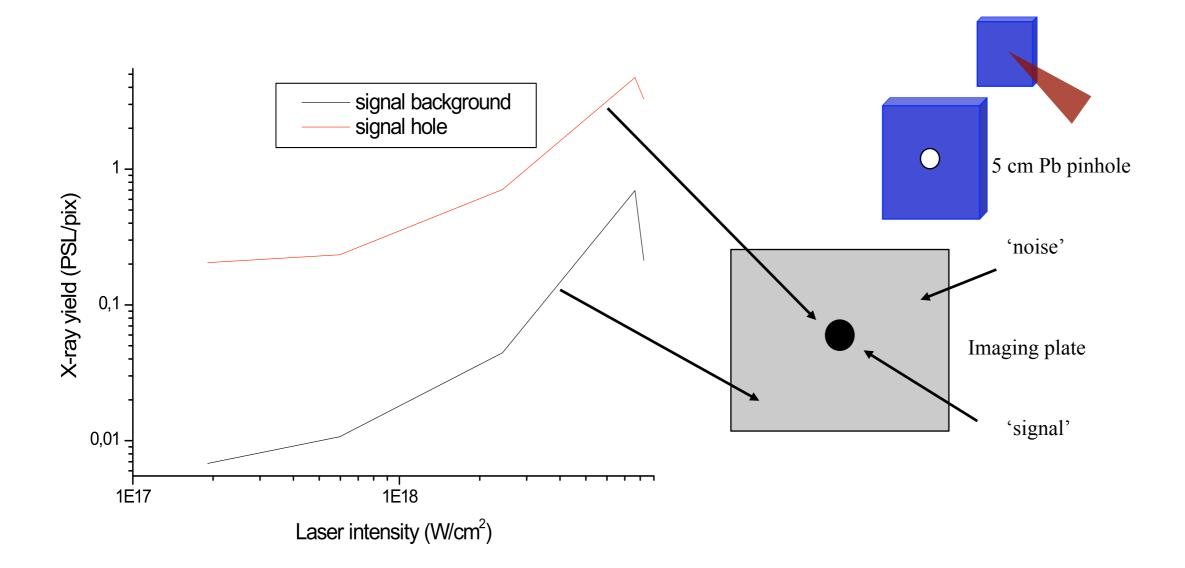
High intensities generate hard x-rays, which penetrate cms of lead (increase faster than signal). Not important for radiography, but for spectrally resolved diagnostics.
