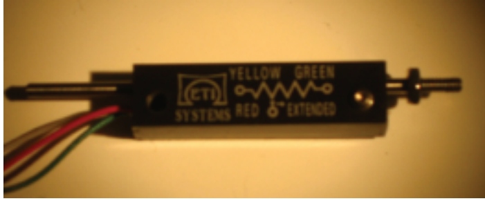
Figure 2.5: Resistor for measuring distance
