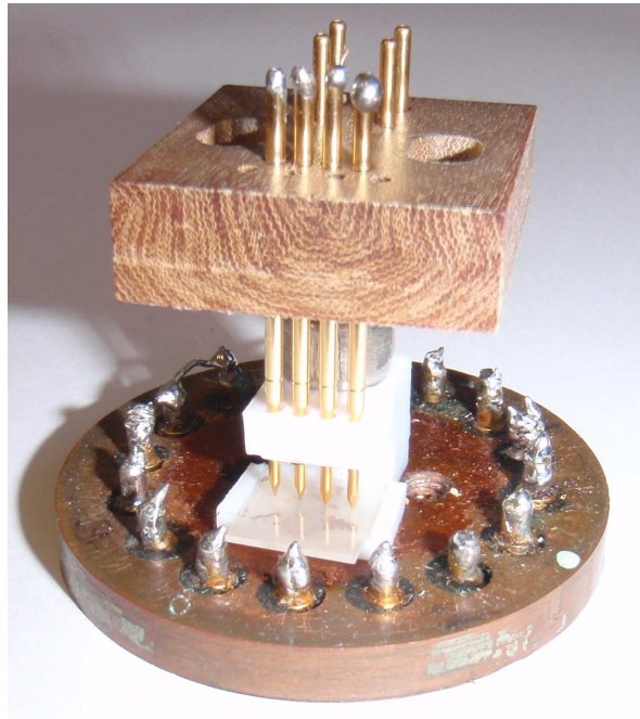
Figure 6.2: The pogo-pin setup used to measure sheet resistance.
