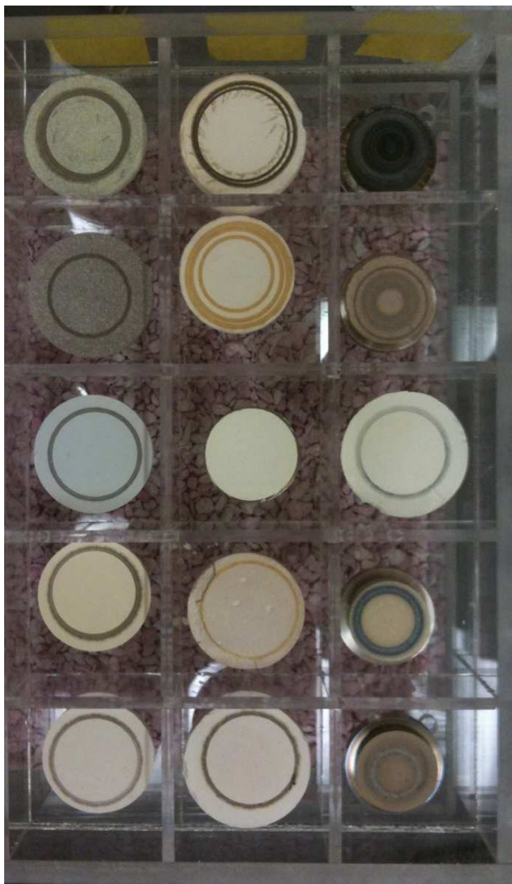
Figure 4.7: Some of the PLD targets that were made using solid state reactions. The rings that can be seen on the surface are where the laser pulse hits the rotating targets.
