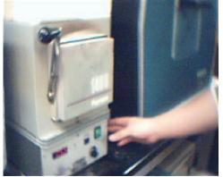
In order to select the  $450^{\circ}$  hold the black button and turn the knob to set the temperature
