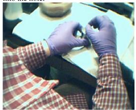
We will scratching very gentle the inner walls of the cylinder pushing the sample that could be stick at the inner surface. Finally we will leave the piston into the cylinder.
