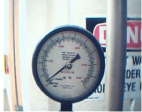
This pressure will be decreasing as the crystals reduce their volume. We will be trying to keep this pressure in 1000lb and ones this pressure remains constant after 2 or 3 min we will remove very slowly the pressure.
