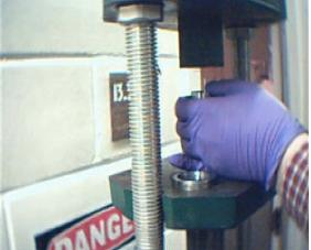
To avoid the piston to fall, we must apply a lateral force to the piston at the same time that we use the press.
