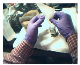
We will use another weighing paper to push any sample left on the top of the cylinder into the hole.
