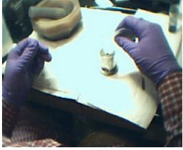
After the entire sample is into the cylinder we will spin the cylinder group the sample inside the cylinder. After this we will procedure to introduce the small cylinder (piston) into the hole.
