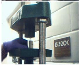
Just when the piston barely is touching the top of the press... we must look for the perfect collocation of the piston. The top surface of the press is not perfectly plane. It makes a small concave surface, so we must make the piston to touch the deepest part of the press.
