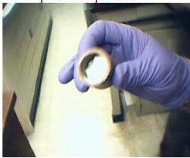
The main idea is to use the press to remove the pill from the cylinder and avoid the piston to fall and damage the pill.
