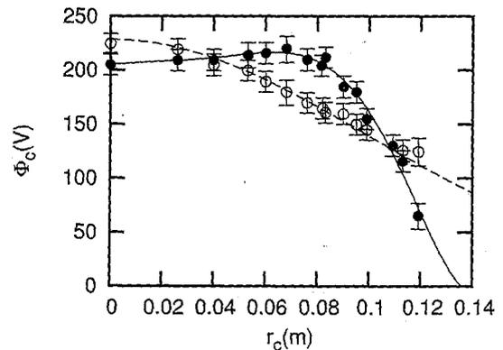
FIG. 2: Radial profile of electrostatic potential in the central cell from Cho *et al.*<sup>3</sup> Filled circles and the solid line represents the experimental data and a parameterized fit, respectively, with the injection of electron cyclotron heating; while hollow circles and the dashed line show results without injection of electron cyclotron heating.
