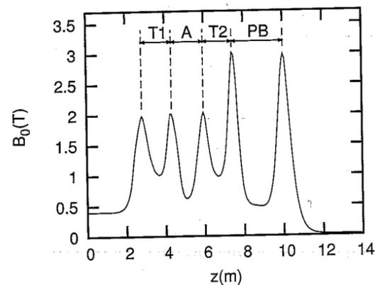
FIG. 1: The axial magnetic field on the right-hand-side of the GAMMA-10 tandem mirror. The central cell of the machine is situated at  $z = 0$  and the left-hand-side of the axial magnetic field is symmetric. Labeled on the figure are transition region 1 (T1), the anchor region (A), transition region 2 (T2) and the plug-barrier region (PB).
