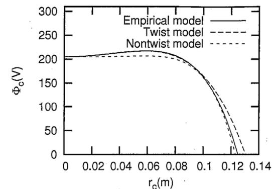
FIG. 3: Three analytic models for electrostatic potential in the central cell constructed from the data of Cho *et al.*<sup>3</sup> in Fig. 2.
