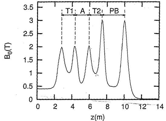
FIG. 1: The axial magnetic field on the right-hand-side of the GAMMA-10 tandem mirror. The central cell of the machine is situated at  $z = 0$  and the left-hand-side of the axial magnetic field is symmetric. Labeled on the figure are transition region 1 (T1), the anchor region (A), transition region 2 (T2) and the plug-barrier region (PB).
