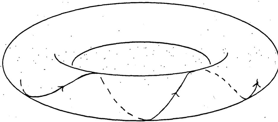
Fig. 4 Tokamak Field Line Configuration
