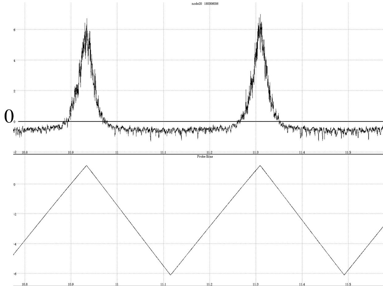
Measure current as applied voltage is swept – here a sawtooth from -60V to 10V with a 0.5 sec period.
