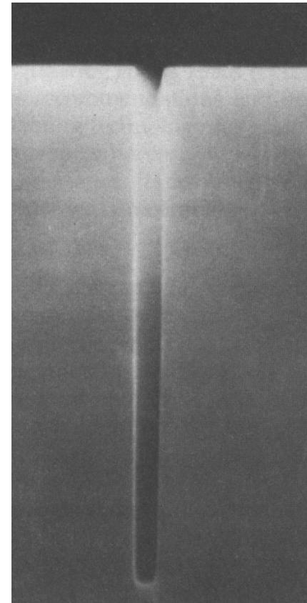
Illustrates sheath at surface that accelerates ions  $\perp$  to surface with energies several times  $T_e$ .
