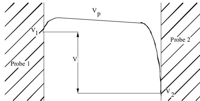
Schematic of potential distribution between the probes of a double floating double-probe
