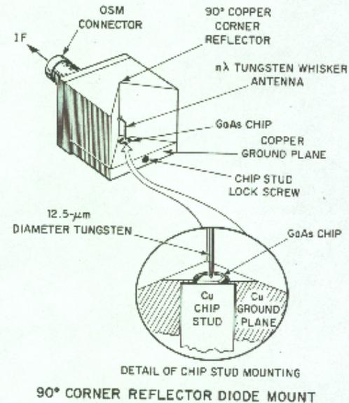
FIG. 31 Schematic of quasi-optical corner reflector Schottky diode mixer (Fetters *et al.*, 1978).
