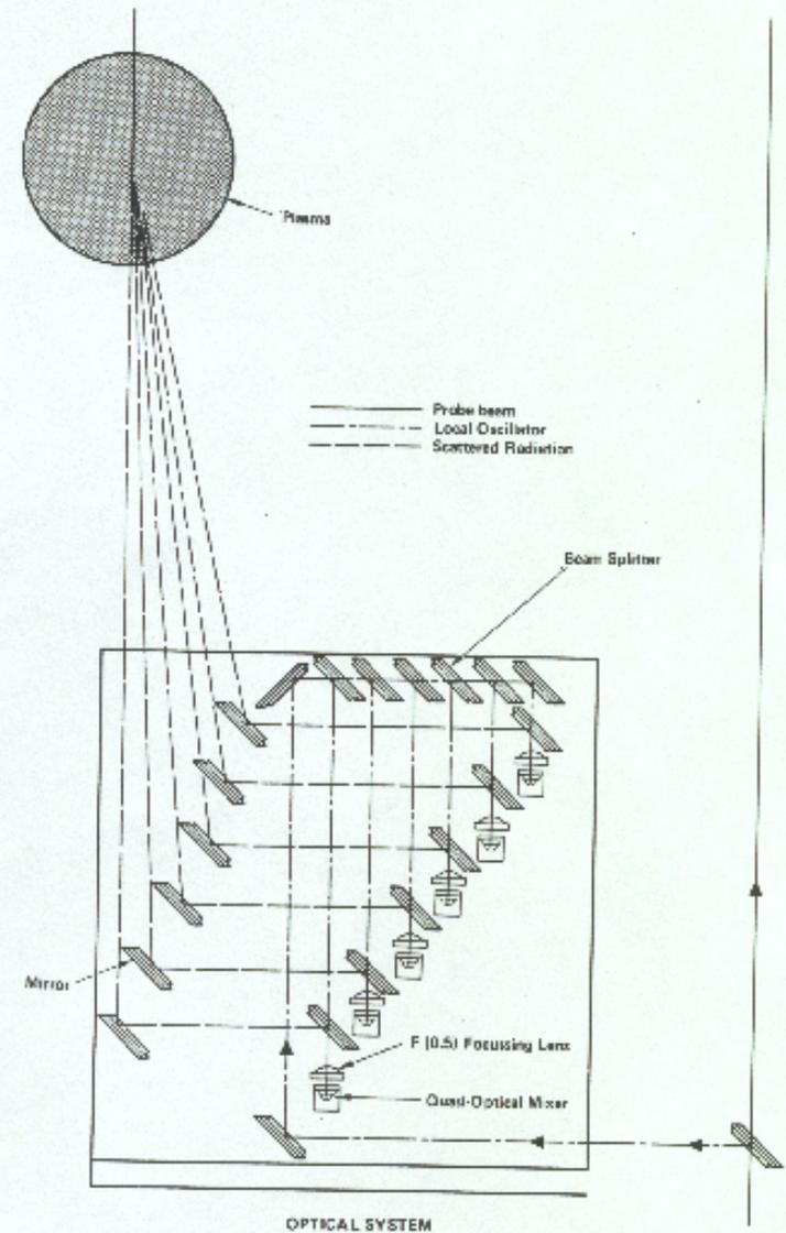
FIG. 39 Multichannel FIR scattering system homodyne receiver schematic.
