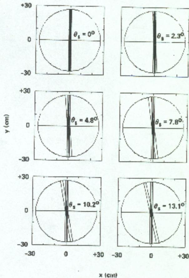
FIG. 20 Scattering volume length versus scattering angle ( $\theta_s$ ) for a source beam at  $\lambda = 1222 \mu\text{m}$ .
