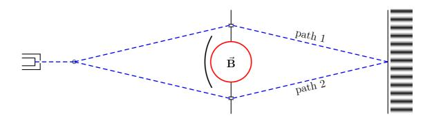
The solenoid is thin, densely wound, and very long, so the magnetic field outside the solenoid is negligible. Inside the solenoid there is a strong **B** field, but the electrons do not go there; instead, they fly outside the solenoid along paths 1 and 2. But despite **B** = 0 along both paths, the magnetic flux  $\Phi$  inside the solenoid affects the interference pattern between the two paths.
