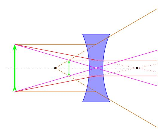
Again, Euclidean geometry tells us that the three refracted rays do not intersect at at a ream image point to the right of the lens, but their extrapolations to the left side do intersect at a virtual image point. Specifically, the virtual image is located at
