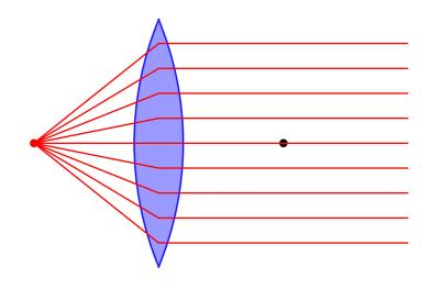
A positive lens can make both real and virtual images, depending on the distance  $d_o$  from the object to the lens: When the distance is greater than the focal length,  $d_o > f$ , the image is real, t when the distance is less than the focal length,  $d_o < f$ , the image is virtual.
