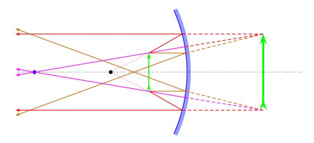
Similar to virtual images in positive lenses, the virtual image in a concave mirror is up-right, its distance  $d_i$  behind the mirror is given by
