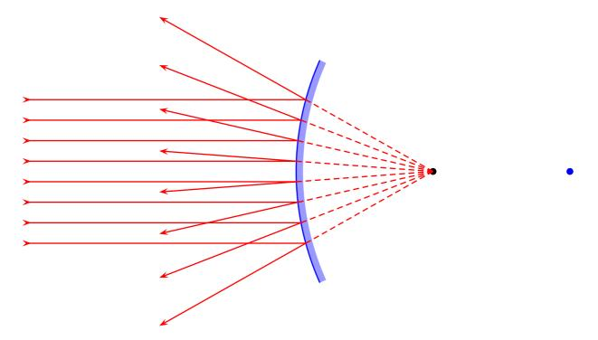
All images in convex mirrors are virtual, up-right, and smaller that the object. Here is the ray diagram:
