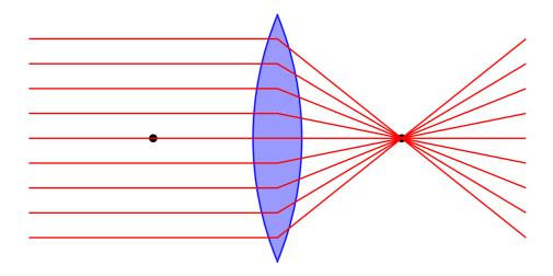
On the other hand, light rays coming out of a focus are refracted so that on the other side of the lens they become parallel:
