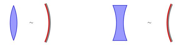
The main difference is that the focal length of a curved mirror is simply a half of the mirror's curvature radius,  $f = \frac{1}{2}R_{\text{curvature}}$ , while the focal length f of a lens has a more complicated dependence of the lens's shape and the refractive index n of the glass (of which the lens is made).
