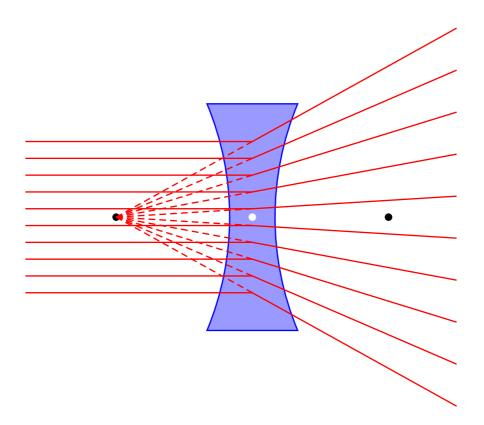
Often, the focal distance of a negative lens is written as a negative number, for example f = -20 cm, where the minus sign indicates that the lens is negative, while 20 cm is the distance from the lens to its virtual focus. In contrast, f = +20 cm would indicate a positive length with real focuses 20 cm from the lens.
