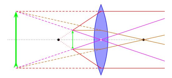
This time, the three rays from each object point do not cross each other on the right side of the lens, but if we extrapolate the refracted rays back to the left side of the lens, they would intersect at the corresponding point of the *virtual image*.
