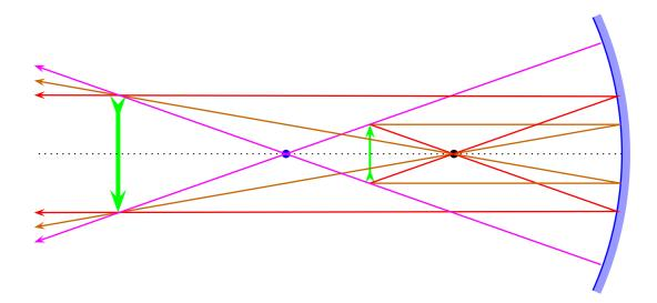
For each interesting point of an object, the first ray (orange) starts parallel to the axis, reflects of the mirror towards the focus, and then continues in a straight line. The second ray (red) goes through the focus to the mirror, the reflects back parallel to the axis. The third ray (purple) goes along the line connecting the object and the center of the mirror; this ray is reflected back towards the center. The three rays intersect at the *real image* located at  $d_i$  such that
