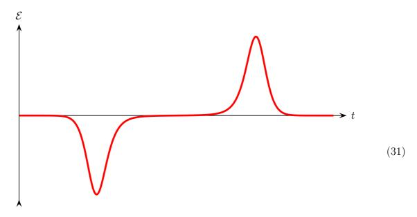
Next, consider the *direction* of the induced EMF. The minus sign in the flux formula (29) encoded the *Lenz rule: The current due to the induced EMF tries to counteract the change*
