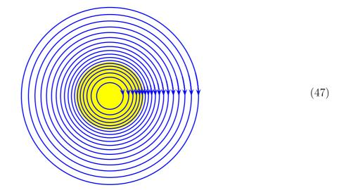
Note that despite the magnetic field being confined to the inside of the solenoid, its timedependence induces the electric field both inside and outside the solenoid (yellow vs. white background on the above picture.)
