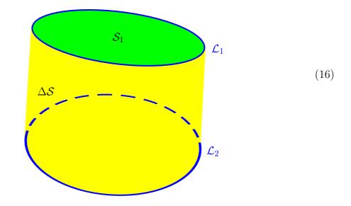
Then the combined surface  $S_2 = S_1 + \Delta S$  spans the loop  $\mathcal{L}_2$ . It might look like a peculiar choice of a surface to span the loop  $\mathcal{L}_2$  at time  $t_2$ , but it does the job. Consequently, the
