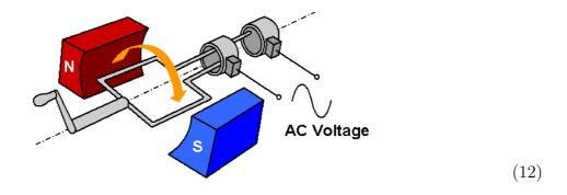
For a simple rectangular loop shown on this picture one may calculate the AC EMF directly from eq. (6), but for more realistic wire coils one has to use eq. (7), and the integral over the moving coil's length can be quite painful to evaluate. Fortunately, there is a much-easier-to-evaluate formula for the motional EMF in terms of the magnetic flux.
