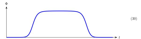
By the Faraday's Law (29), this flux produces two pulses of EMF, first a negative pulse when the magnet enters the loop, and then a positive pulse when the magnet exits,
