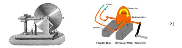
A conducting disk is rotated around its axis with angular velocity  $\omega$ , so a part of the disk at distance s from the axis moves at velocity  $\mathbf{v} = \omega s \hat{\phi}$ . In a magnetic field parallel to the axis, this makes for
