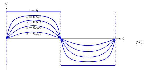
Note: the closer we are to the axis the smaller is the amplitude of the  $V(\phi)$  curve the more the curve looks like the sine wave. The mathematical reason is that all non-constant terms in the
