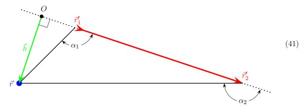
Since the wire segment is straight, the infinitesimal vector  $d\vec{\ell} = d\mathbf{r}'$  along the segment has a fixed direction, same as  $\mathbf{r}'_2 - \mathbf{r}'_1$ . Consequently, the vector product in the numerator of the BSL integral remains constant along the whole segment. Indeed,
