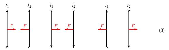
Here is the graphical explanation of the force's direction for the currents in the same direction:
