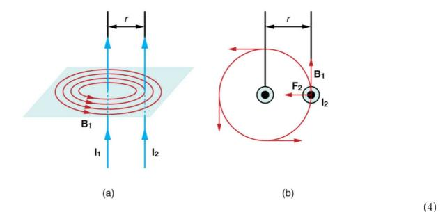
The magnitude of the force between two wires per unit of wire's length is
