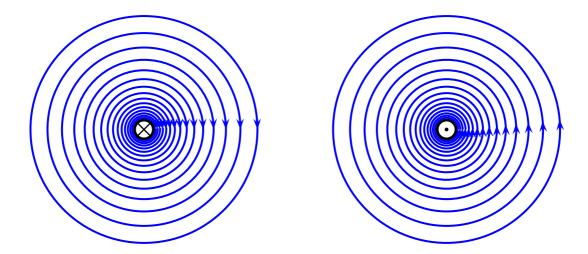
The effect of this magnetic field on another long wire parallel to the first wire is an attractive force if the currents in the two wires flow in the same direction, and a repulsive force if the
