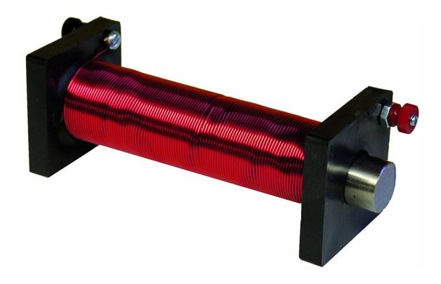
To simplify the calculation of the magnetic field created by this solenoid, let's assume its length is much longer than its diameter, so to a first approximation we may treat it as infinitely long, hence the cylindrical symmetry. By this symmetry (and also by the reflection  $z \to -z$  symmetry), the magnetic field everywhere — both inside and outside the solenoid — points in z direction while its magnitude depends only on s. Furthermore, by the Ampere Law applied to the  $\mathbf{H}$  field,
