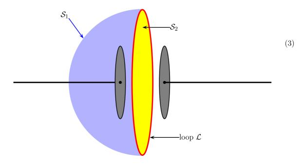
Of course, the current does not really flow *through* the capacitor but only through the wires connected to each of the capacitor's plates. Inside the capacitor, there is no electric current; instead, the charges temporarily accumulate on the plates according to
