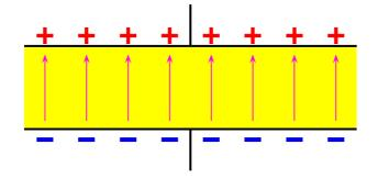
Let d be the distance between the plates and A the plates' area. Given the voltage V between the capacitor plates, the electric field inside the capacitor is approximately uniform
