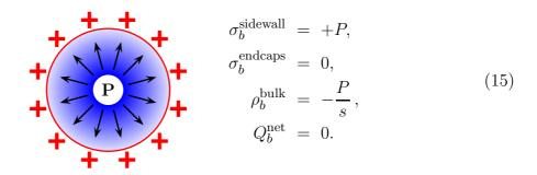
In fact, for any dielectric geometry and any polarization field, uniform or not, the net bound charge is zero since the bound charges cannot in or out of the dielectric. Indeed,
