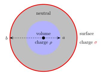
Find the electric in each of the three regions: (i) r < a, inside the inner cylinder; (ii) a < r < b, inside the outer shell; (iii) r > b, outside the cable. Plot  $|\mathbf{E}|$  as a function of the radius r.
