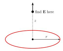
**Problem 2.6:** Find the electric field at height z directly above the center of a flat circular disk of radius R that carries a uniform surface charge  $\sigma$ .
