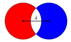
Show that the electric field in the overlapping region is uniform and calculate its value as a function of the vector  $\mathbf{d}$  from the positive center to the negative center.
