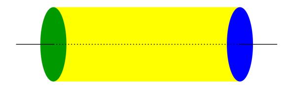
However, on the endcaps the electric field (24) lies parallel to the endcaps instead of crossing them, so the flux through the endcaps is zero. Instead, the entire flux comes through the
