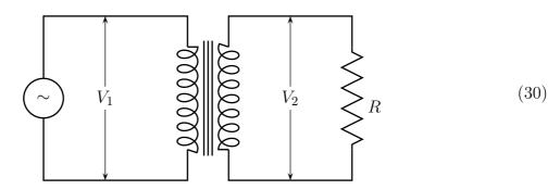
There are AC currents  $I_1(t)$  and  $I_2(t)$  flowing through the respective coils, and the mutual inductions  $M_{21}$  and  $M_{12}$  of the two coils — as well as their self-inductions  $L_1$  and  $L_2$  — give rise to the EMFs in both coils. Specifically,
