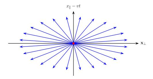
In the limit of ultra-relativistic charge velocity — v so close to c that  $\gamma \gg 1$ , — this picture becomes so squashed that the fields are pretty much limited to the transverse plane
