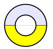
Note: the boundary between the dielectric and the vacuum lies in the same plane as the common center of the two spheres.
