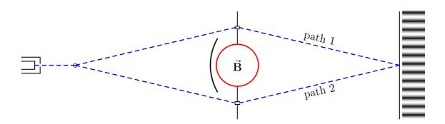
The solenoid is thin, densely wound, and very long, so the magnetic field outside the solenoid is negligible. Inside the solenoid there is a strong  $\mathbf{B}$  field, but the electrons do not go there; instead, they fly outside the solenoid along paths 1 and 2. But despite  $\mathbf{B} = 0$  along both paths, the magnetic flux  $\Phi$  inside the solenoid affects the interference pattern between the two paths.
