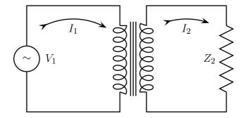
For simplicity, consider an ideal transformer: perfectly linear ferromagnetic core with no hysteresis, no eddy currents in the core, no ohmic losses in the wiring of the coils, and perfect magnetic coupling of the two coils, k = 1.
