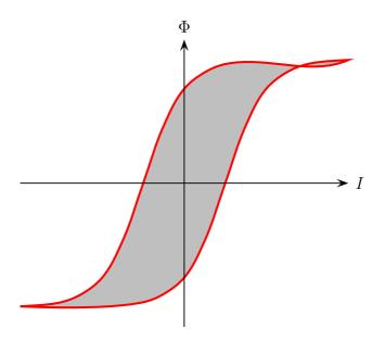
and this net work is dissipated as heat rather than stored as magnetic energy.
