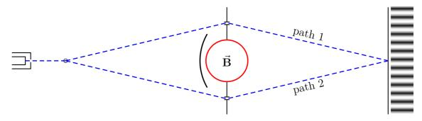
The solenoid is thin, densely wound, and very long, so the magnetic field outside the solenoid is negligible. Inside the solenoid there is a strong **B** field, but the electrons do not go there; instead, they fly outside the solenoid along paths 1 and 2. But despite  $\mathbf{B} = 0$  along both paths, the magnetic flux F inside the solenoid affects the interference pattern between the two paths.
