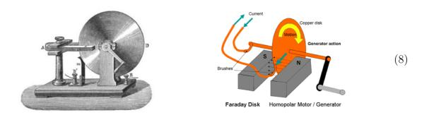
A conducting disk is rotated around its axis with angular velocity  $\omega$ , so a part of the disk at distance s from the axis moves at velocity  $\mathbf{v} = \omega s \,\hat{\phi}$ . In a magnetic field parallel to the axis, this makes for
