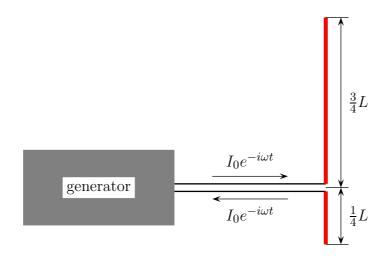
For simplicity, approximate the current in the antenna by a sine wave with nodes at both ends, thus
