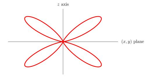
Surprisingly, there are 2 major lobes, one centered at  $\theta = 58^{\circ}$  and the other at  $\theta = 122^{\circ}$  — i.e.,  $32^{\circ}$  above or below the horizontal, — while no radiation is emitted in the horizontal or vertical direction.
