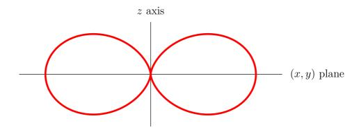
For the short dipole antenna, this radiation pattern diagram has a single main lobe centered at the horizontal plane, but this main lobe is rather thick, so a lot of radiation goes in directions well above or well belows the horizontal.
