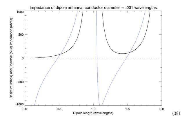
The black line on this plot shows the input resistance  $R_{\rm in}$  — *i.e.*, the real part of the input impedance  $Z_{\rm in}$  — of a center-fed linear antenna as a function of  $L/\lambda$ . The net power radiated by the antenna is related to this resistance as
