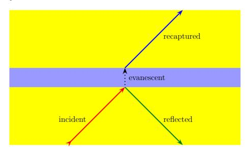
An indirect consequence of the evanescent wave is the Goos–Hänchen effect: In a total internal reflection, the reflected ray is displaced sideways relative to the incoming ray as if it's reflected not from the boundary itself but from a small distance behind it.
