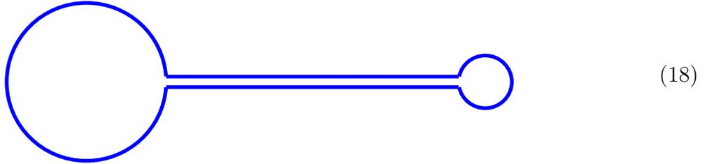
Since the total flux through both loops is quantized, it cannot be changed adiabatically. Therefore, small adiabatic changes of the magnetic field going through the big loop result in much bigger changes of the field in the small loop. The amplification factor is given by (minus) the area ratio.
