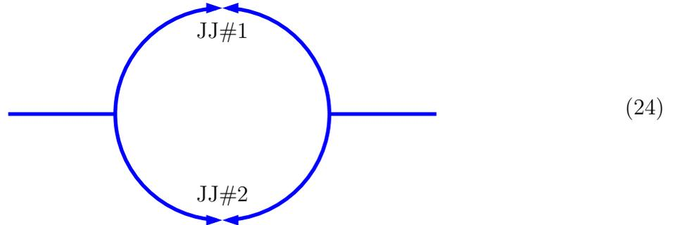
In the absence of magnetic field, the maximal supercurrent that can flow through a symmetric SQUID is clearly  $2I_0$ ; in the presence of magnetic field things are much more interesting.
