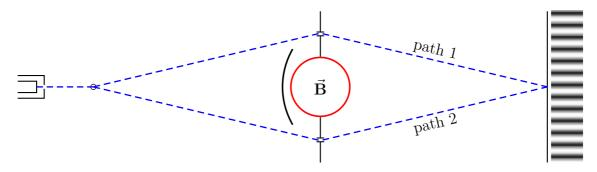
The solenoid is thin, densely wound, and very long, so the magnetic field outside the solenoid is negligible. Inside the solenoid there is a strong  $\mathbf{B}$  field, but the electrons do not go there; instead, they fly outside the solenoid along paths 1 and 2. But despite  $\mathbf{B} = 0$  along both paths, the magnetic flux F inside the solenoid affects the interference pattern between the two paths.
