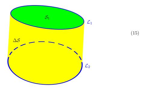
The combined surface  $S_2 = S_1 + \Delta S$  spans the loop  $\mathcal{L}_2$ ; it might look like a peculiar choice of a surface to span the loop  $\mathcal{L}_2$  at time  $t_2$ , but it does the job. Consequently, the magnetic flux at time  $t_2$  can be calculated using this surface, thus
