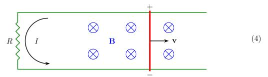
The wire's velocity adds to the velocities of the conducting electrons relative to the wire,
