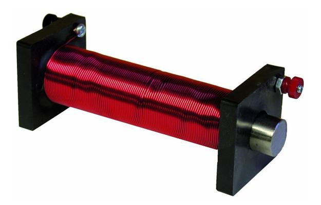
To simplify the calculation of the magnetic field created by this solenoid, let's assume its length is much longer than its diameter, so to a first approximation we may treat it as infinitely long, hence the cylindrical symmetry. By this symmetry (and also by the reflection  $z \rightarrow -z$  symmetry), the magnetic field everywhere — both inside and outside the solenoid — points in z direction while its magnitude depends only on s. Furthermore, by the Ampere Law applied to the **H** field,
