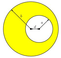
A current of uniform density **J** flows along this conductor in the direction +z (out from the page into your face).
