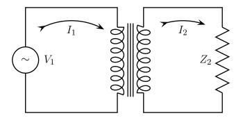
For simplicity, consider an ideal transformer: perfectly linear ferromagnetic core with no hysteresis, no eddy currents in the core, no ohmic losses in the wiring of the coils, and perfect *magnetic coupling* of the two coils, k = 1.
