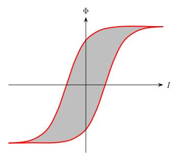
and this net work is dissipated as heat rather than stored as magnetic energy.
