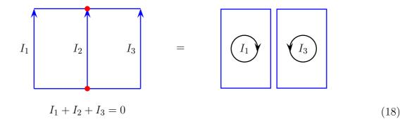
And since both the Biot-Savart-Laplace formula and the magnetic force formula are linear, the net magnetic force between the two circuits is simply the sum of forces between the current loops comprising the two circuits,
