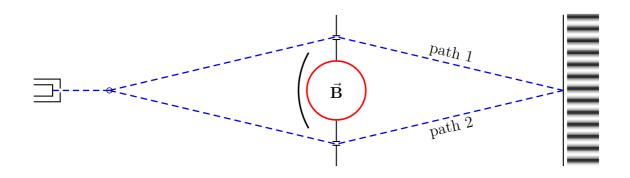
The solenoid is thin, densely wound, and very long, so the magnetic field outside the solenoid is negligible. Inside the solenoid there is a strong **B** field, but the electrons do not go there; instead, they fly outside the solenoid along paths 1 and 2. But despite  $\mathbf{B} = 0$  along both paths, the magnetic flux  $\Phi$  inside the solenoid affects the interference pattern between the two paths.
