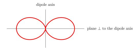
Note: the radiation is strongest in the directions  $\perp$  to the dipole axis, weaker in other directions, and there is no radiation at all in the direction of the dipole axis itself. For example, a vertical antenna has vertical dipole moment  $\mathbf{p}$ , hence the radiation is strongest in the horizontal direction, weaker in directions at some angles above or below the horizon, and no radiation at all goes vertically up or vertically down.
