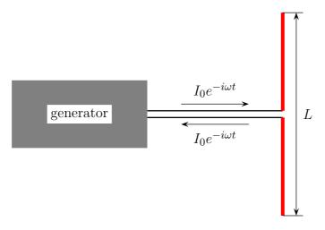
Neglecting the antenna's thickness, we can write the current in the antenna as
