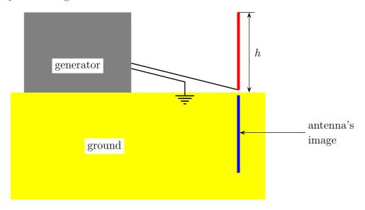
The ground acts as a good conductor, so the charged antenna above the ground is accompanied by its mirror image (of the opposite charge) below the ground. Together, the antenna and its image act as a combined center-fed dipole antenna of net length L=2h, hence the dipole moment amplitude
