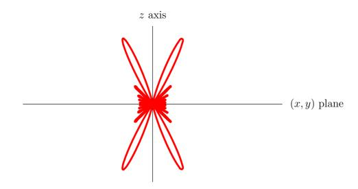
\* In general, the radiation pattern diagram for an antenna of length  $L = n\lambda$  for some integer n has n lobes centered at angles  $\theta$  which obtain from the transcendental equation
