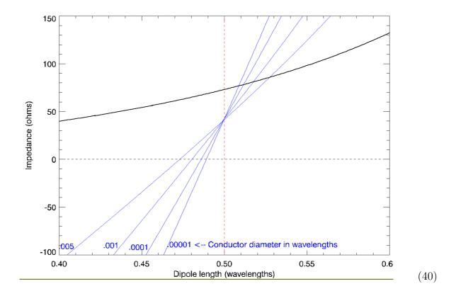
Curiously, for antenna of length exactly  $\frac{1}{2}\lambda$ , the reactance seems to be diameter-independent
