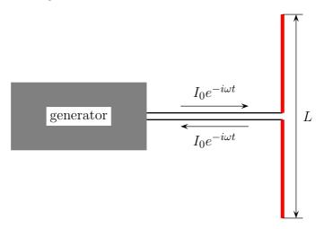
For simplicity, let's assume the antenna's diameter is negligibly thin compared to the antenna's length, so we may approximate the current in the antenna as
