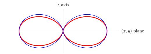
The thin blue line here is for comparison purposes: it's the radiation pattern diagram for a short-dipole antenna. We see that both radiation patterns have a single main lobe centered in the horizontal plane, bot for the half-dipole antenna this main lobe is not quite as thick as for the short-dipole antenna.
