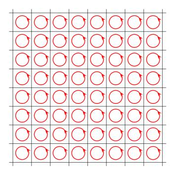
The red loops here stand for the current loops creating the atomic magnetic moments **m**. We do not know the radii or even the shapes of these loops or the currents which flow through
