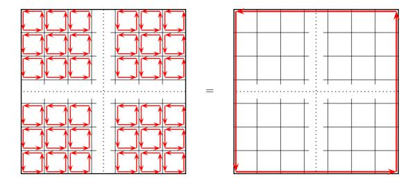
Instead, there is un-canceled current  $I=m/a^2$  flowing counterclockwise around the entire outer boundary of the crystal, or rather of single atomic layer of the crystal. The next layer on top of the layer shown on the above picture has a similar current, and so is every other layer, which makes for a surface current density
