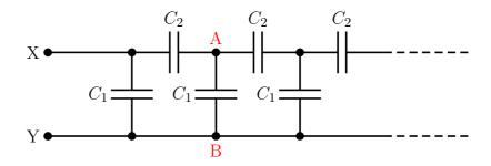
The key to solving this circuit is its very infinity, which means that the sub-circuit comprising everything to the right of the first capacitor pair — *i.e.*, everything to the right of points A and B — is completely equivalent to the whole circuit. Consequently, the equivalent capacity of the complete circuit between points X and Y is equal to the equivalent capacity of the subcircuit to the right of A and B,
