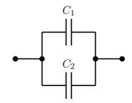
The currents through the two capacitors are separate so they acquire separate charges  $Q_1$ and  $Q_2$ . Moreover, when the capacitors discharge, their charges flow separately through the outside wires, thus
