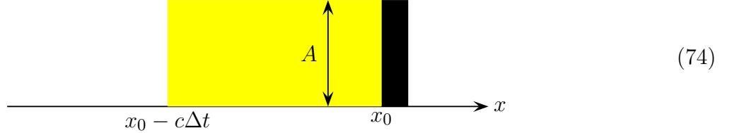
During time  $\Delta t$ , the fields initially located in this volume would travel to the absorber and disappear, while the net momentum of these fields
