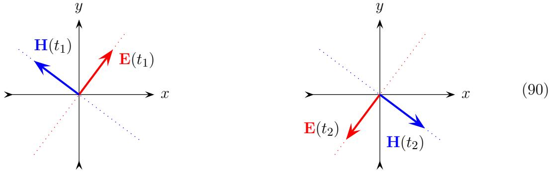
Note: on this diagram, the  $+z$  direction of the wave is towards your face, that's why the magnetic field points 90° to the left the electric field. If you were looking at the field from the opposite direction of the wave's source, the magnetic field would point 90° to the *right* of the electric field. [This web page](#) has an animated 3D diagram that clarifies the relative directions of the two fields.
