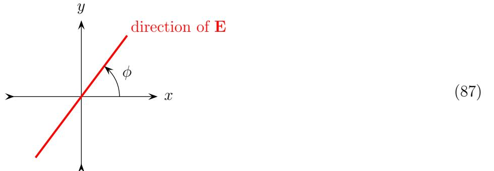
That's why such polarizations are called *linear*. The same polarizations are called *planar* after the shape of the 3D plot of the electric wave  $\mathbf{E}(z)$  (for any fixed time  $t$ ): Such a plot is restricted to a single 2D plane, spanning the  $z$  axis and the red line on the above diagram, for example [this plot](#).
