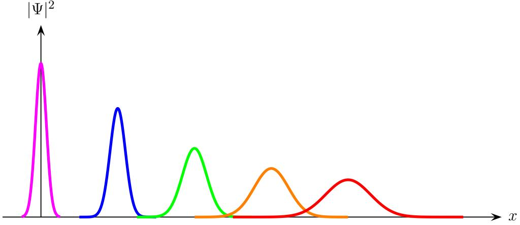
The dispersion limits the pulse rate — and hence the information transfer rate — in long transmission lines, from 19<sup>th</sup> century telegraph cables to modern fiber optic cables. Indeed, whatever the initial pulse width  $a$ , by the time the pulse reaches the end of the line at time  $T = L/v_g$ , its width  $\Delta x(T)$  must be shorter than the space interval between the pulses, or else we would not be able to resolve them from each other. In terms of the pulse rate
